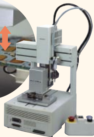
Cycling fatigue test of mounted PCB
