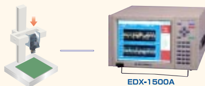
Drop impact test of mounted PCB
